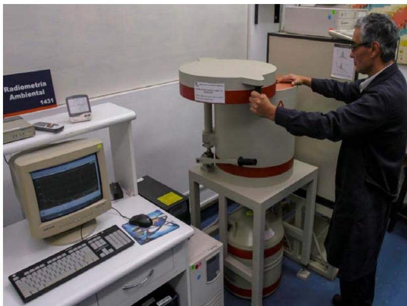
**Figure 3.** Gamma spectrometry system.
